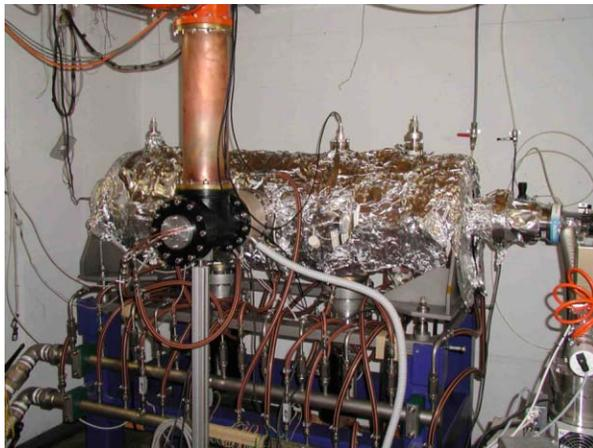
Figure 2: The 5-cell cavity in the lab test stand.
