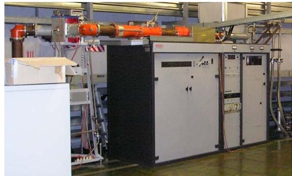
Figure 3. The power amplifier and the circulator.
