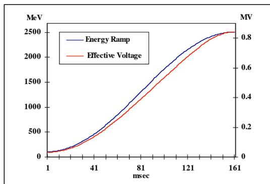
Figure 1: Voltage and beam energy ramps.
