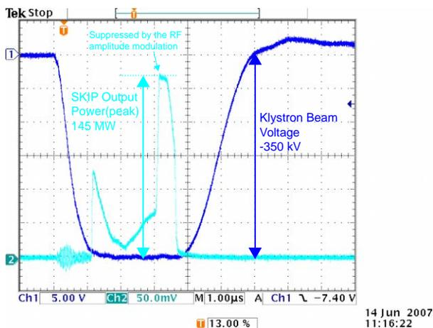
Figure 4: Ch1: RF output power from the SKIP. Ch2: Klystron beam voltage.
