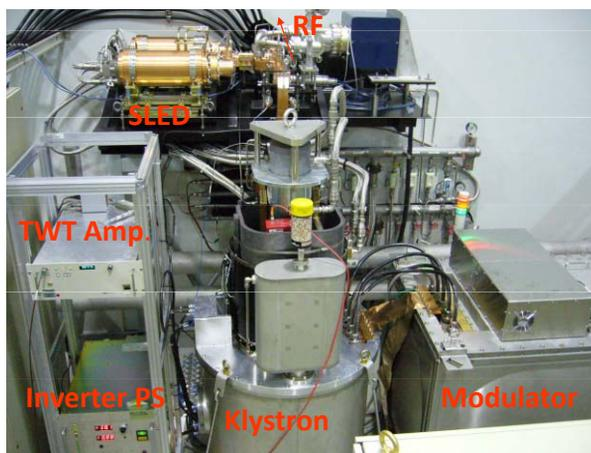
Figure 2: A photograph of the C-band RF source.
