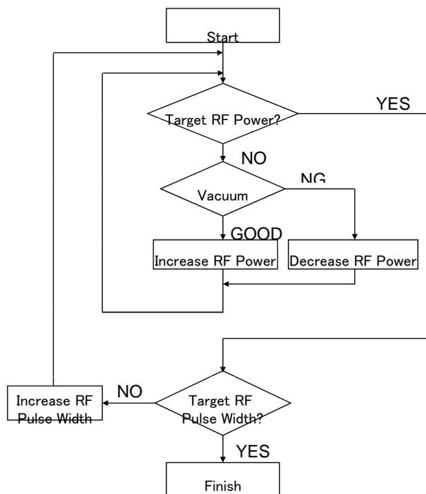
Figure 3: A flow chart of the RF processing. The RF power is controlled by changing the charging voltage of the inverter power supply.
