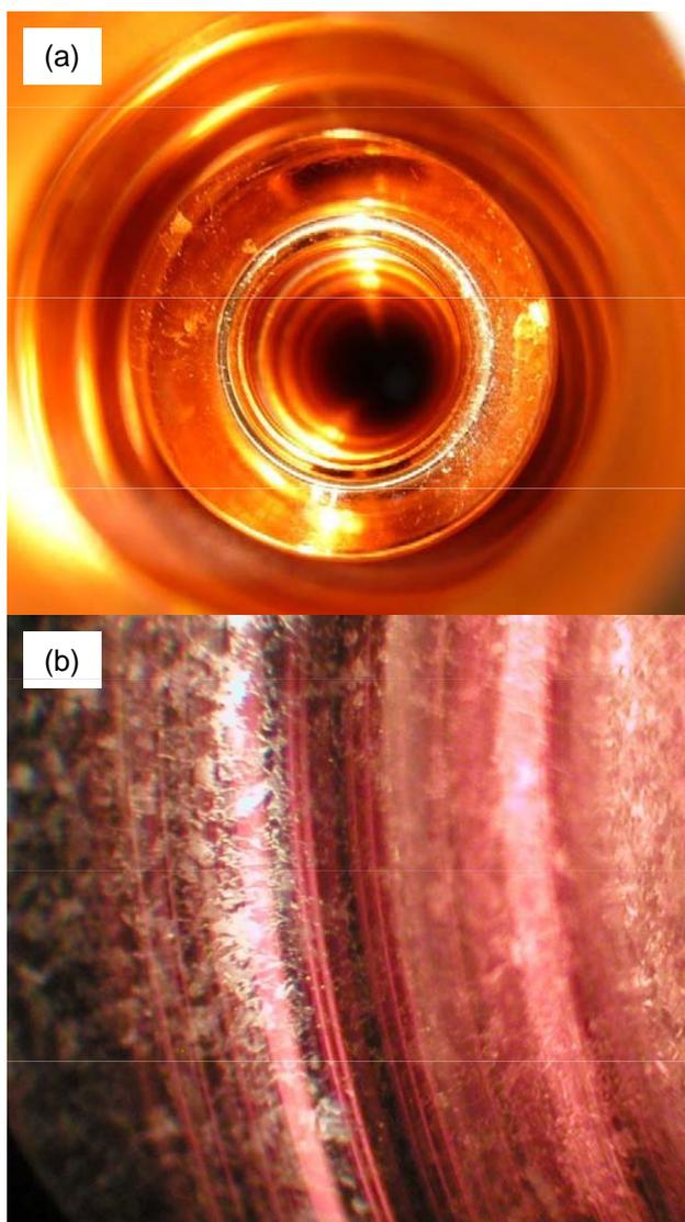
Figure 5: (a) Inside view of the C-band accelerating structure. (b) The upstream iris edge observed with the borescope. The small difference of the surface color shows the grain boundary of Cu.
