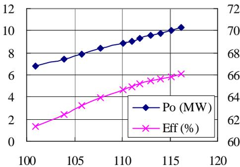
Figure 5: The measured output power and efficiency as a function of the beam voltage.
