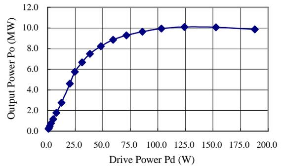
Figure 6: The transfer curve at the beam voltage of 115kV.
