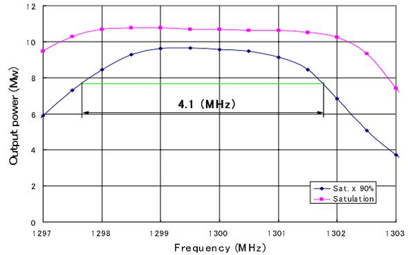
Figure 7: The instantaneous bandwidth both at saturation and 90% of saturation.
