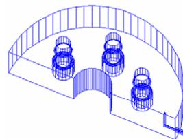
Figure 3: Cross section of an input cavity.
