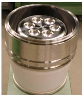
Figure 2: Electron gun of the E3736 MBK.
