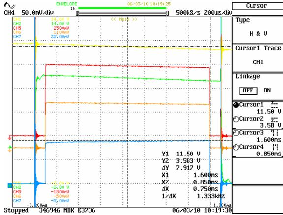
Figure 4: Waveforms. Cathode voltage (115kV, 1.7ms-long, yellow), collector current (133A, 1.7ms-long, green), RF output from the two ports (10.2MW in total, 1.5ms-long, red and orange).
