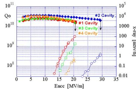
Figure 4: Qo vs. Eacc curves and x-ray radiation level in the final performance on four STF-Baseline cavities.
