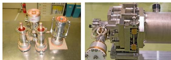
Figure 2: Input couplers and a slide-jack tuner system.
