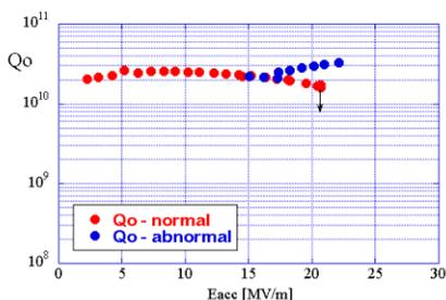
Figure 7: Strange behaviour of Qo values due to the excitation of the 8π/9 passband mode inside the cavity.
