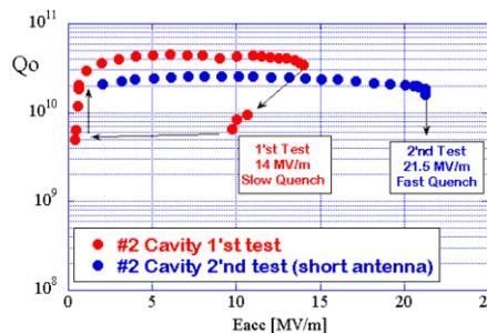
Figure 8: Degradation of Qo values due to heating at the HOM pickup antenna.
