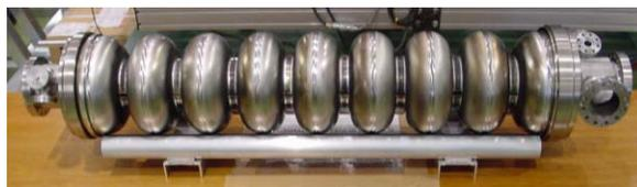
Figure 1: The STF Baseline 9-cell Cavity.
