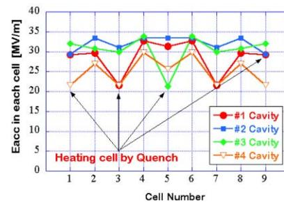
Figure 5: Achievable Eacc in each cell for four cavities.
