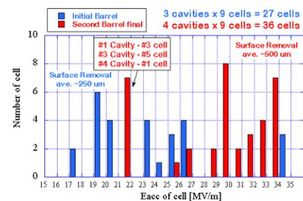
Figure 6: Distribution of the achievable Eacc in each cell before and after the 2<sup>nd</sup> barrel polishing.
