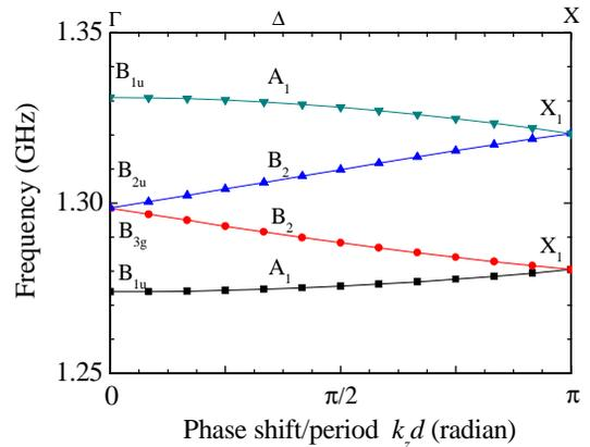
Figure 3: A dispersion relation of the side-coupled structure. Only the lowest passband is shown.
