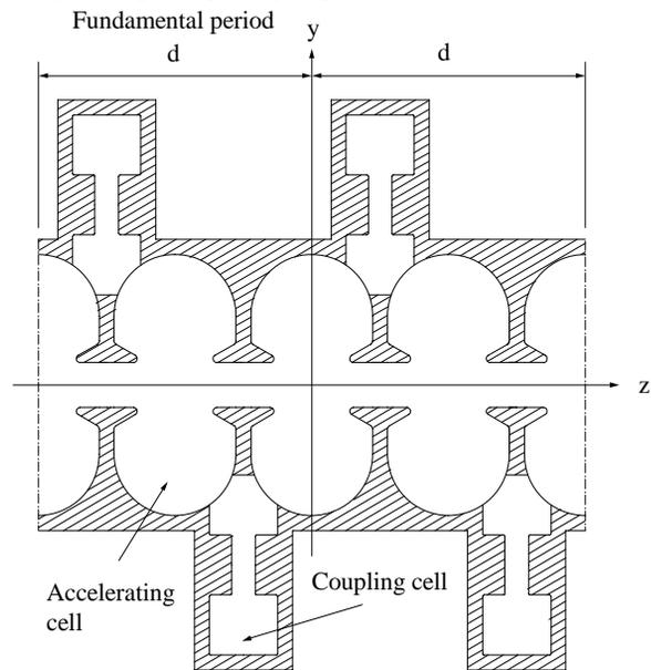
Figure 1: A sketch of the side-coupled structure.
