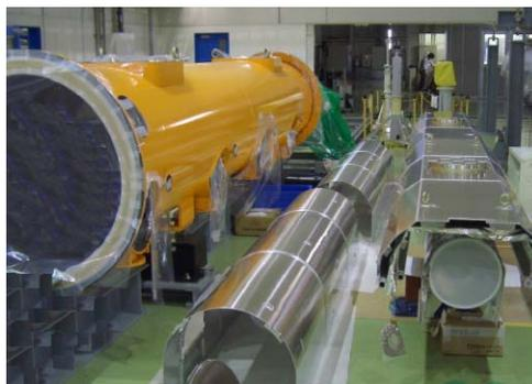
Figure 4: Components of STF cryostat
