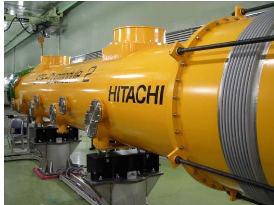
Figure 8: Completed STF cryomodule
