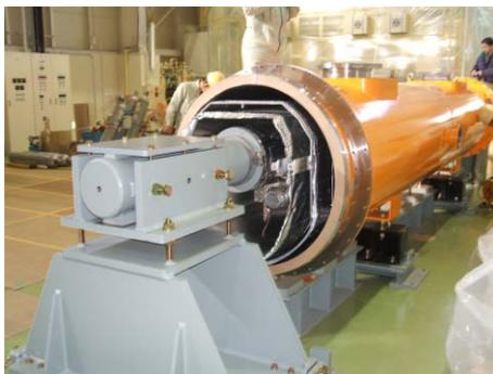
Figure 7: Insertion into the vacuum vessels
