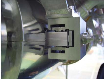
Figure 6: Cavity sliding fixtures
