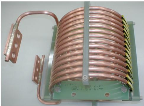
Figure 8: 14-turn inductor production version
