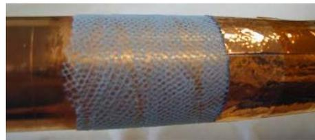
Figure 10: Polyethylene mesh as an extra spacer.
