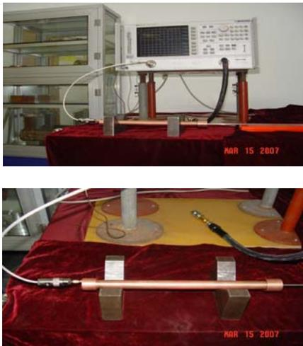
Figure 2: The measurement system of the permeability.
