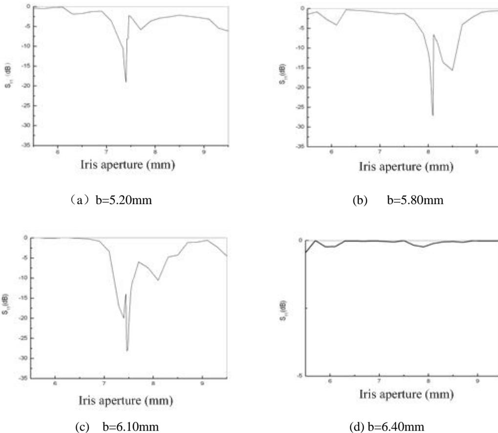
Figure 3: The calculated values of  $S_{11}$  vs the coupler widths
