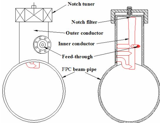
Figure 2: PEFP HOM coupler and cross-section on FPC beam-pipe.
