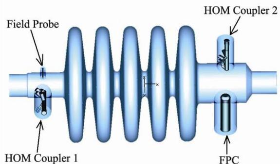
Figure 5: A 3-D MWS mode of a PEFP low-beta cavity with two HOM couplers, an FPC and a Field Probe.
