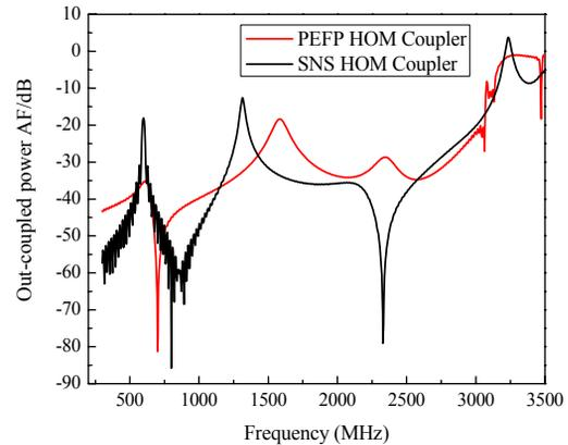
Figure 4: Out-coupled power comparison between a PEFP HOM coupler and an SNS HOM coupler.
