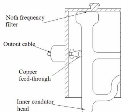
Figure 1: A SNS HOM Coupler schematic [5,6].
