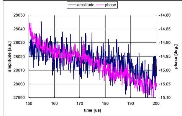
Figure 4: RF amplitude and phase in DTL cavity.
