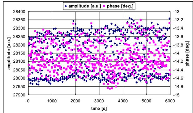
Figure 5: Pulse-to-pulse stability measurement results.
