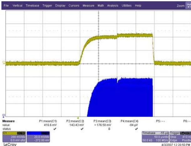
Figure 3(c): Feedback control with Feed-forward. (upper: Forward RF power, lower: Cavity field).
