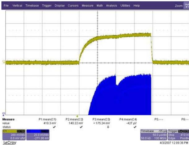
Figure 3(b): Cavity field response for feedback control. (upper: Forward RF power, lower: Cavity field).
