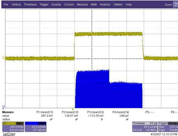
Figure 3(a): Cavity field response for Open-Loop Case. (upper: Forward RF power, lower: Cavity field).
