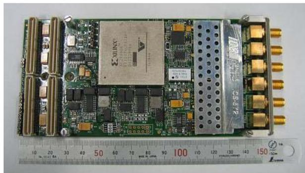
Figure 1: ICS-572B PMC Board.
