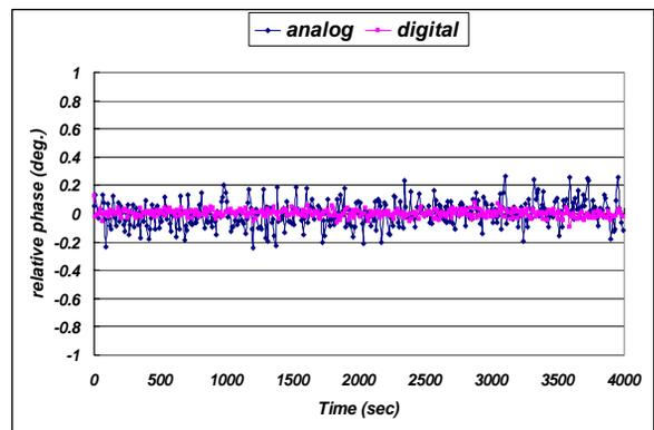
Figure 5: Relative phase measured between two cavities.
