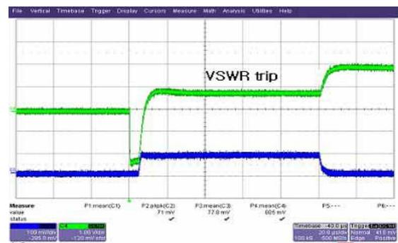
Figure 2: VSWR trip signal measured in the HPRF test.
