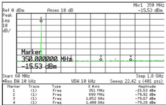
Figure 3: Output frequency response of analog chassis.
