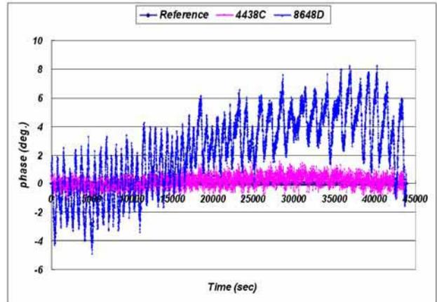
Figure 4: Phase stability of RF signal generators.
