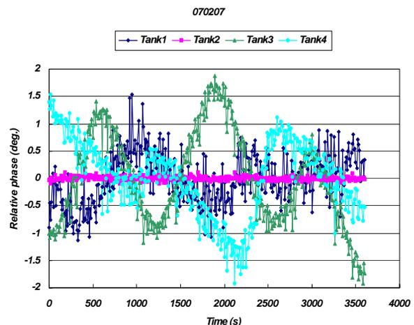
Figure 6: Relative phase measured in the HPRF test for the DTL.
