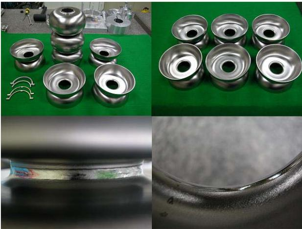
Figure 5: Welding surface of iris part
