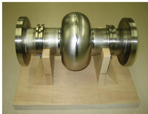
Figure 3: 3<sup>rd</sup> harmonic SRF cavity for PLS
