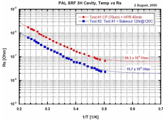
Figure 4: Surface resistance with temperature
