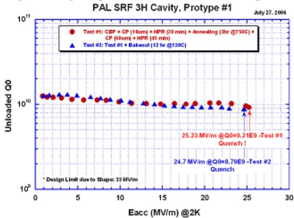
Figure 5: Measured accelerating electric field and  $Q_0$
