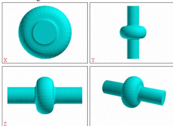
Figure 1: 3D model of 3H SRF cavity
