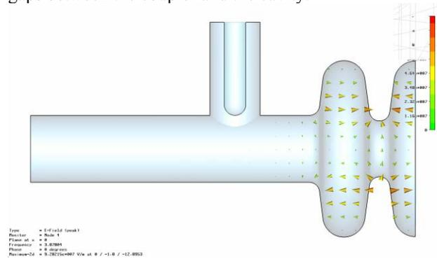
Figure 1: Microwave Studio simulations of a 3-cell cavity.
