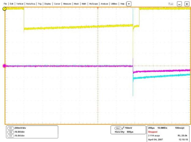
Figure 5: CCII Quench at low (16 MV/m) gradient. Yellow – Forward power, Magenta – Downstream Faraday Cup, Cyan – Upstream Faraday Cup.
