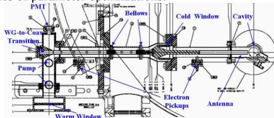
Figure 2: Layout of the 3.9 GHz power coupler.
