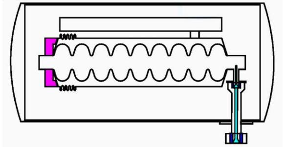
Figure 12: Model of the horizontal test cryostat.
