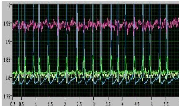
Figure 10: Fast thermometry shows quench in the bottom cell in “8Pi/9” modes at 120 mT surface cell.
