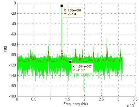
Figure 4: 14-bit ADC SNR
