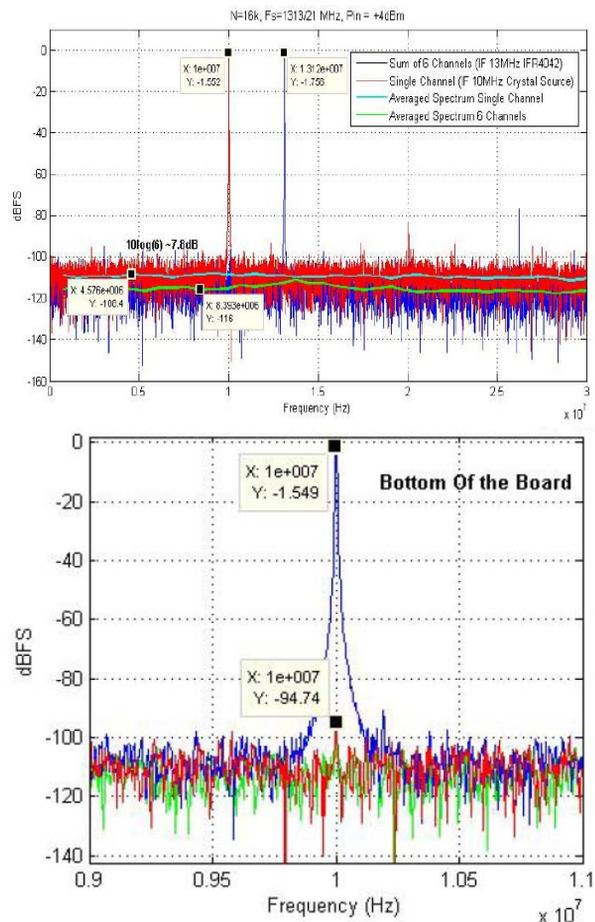
Figure 5: 8 ch ADC - Process gain and Crosstalk
