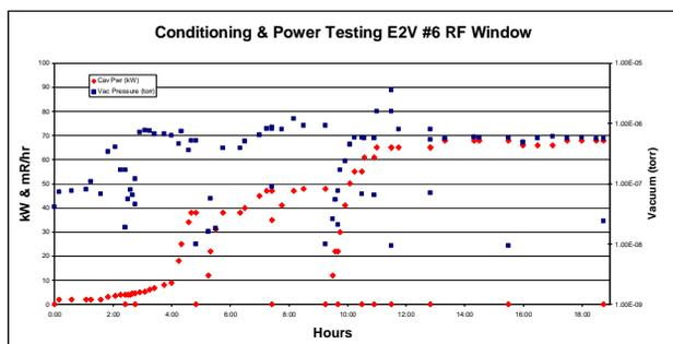
Figure 4: RF window E2V-6 power conditioning.
