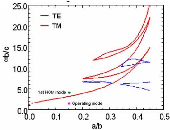
Figure 2: Plots of global band gaps for TM and TE modes as functions of  $a/b$  as obtained from PBG calculations for the triangular lattice in Fig.1.
