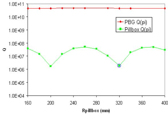
Figure 4: Plot of  $Q$  as a function of the coupler radius for the pillbox coupler and the PBG HOM coupler.
