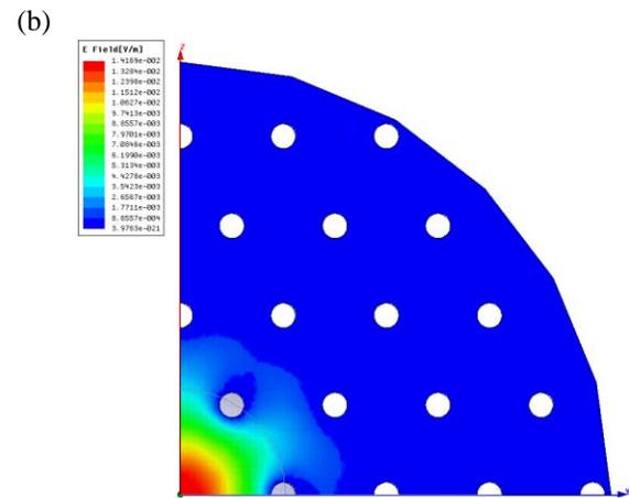
Figure 3: (a) 2-cell model with two TESLA cavities and two PBG HOM coupler; (b) the operating mode structure with a frequency of 1.293 GHz in the transverse plane of the PBG HOM coupler.
