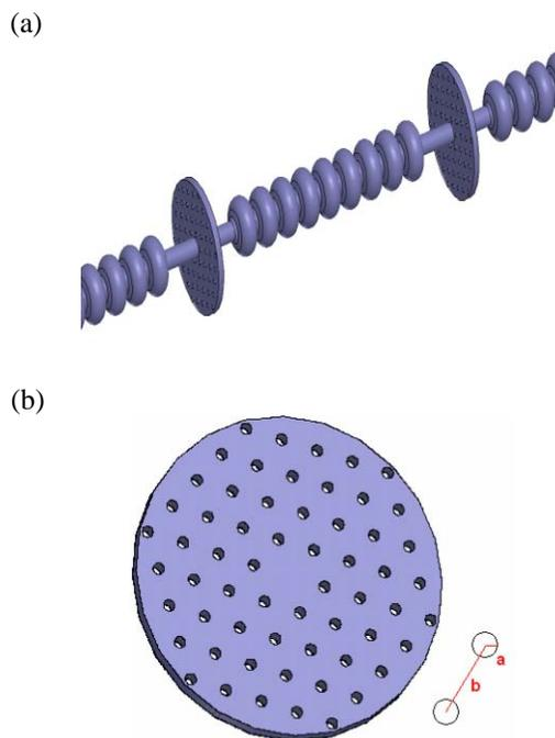
Figure 1: (a) Schematic layout of the PBG HOM coupler and (b) triangular superconducting PBG lattice design with  $a = 8.25$  mm and  $b = 55$  mm.
