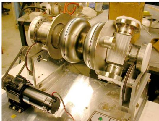
Figure 6: 1-cell/2-cell cavity tumbling apparatus.
