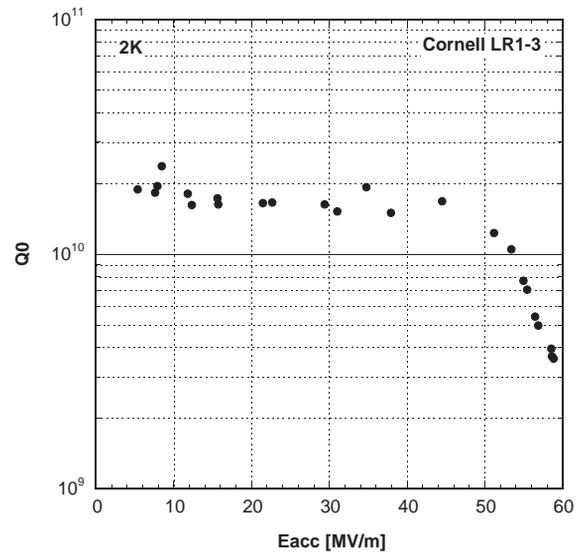
Figure 3:  $Q_0(E_{acc})$  of the 60 mm aperture single-cell cavity LR1-3.
