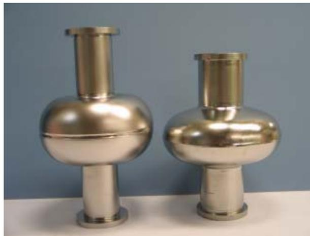
Figure 1: Left: 60 mm aperture re-entrant cavity; Right: 70 mm aperture TESLA cavity.
