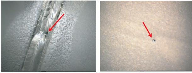
Figure 2: Defect at the EBW overlap of the equator joint of LR1-4. Left: before repair; Right: during repair with CBP after 50  $\mu\text{m}$  surface removal. Photo credit: T. Saeki.
