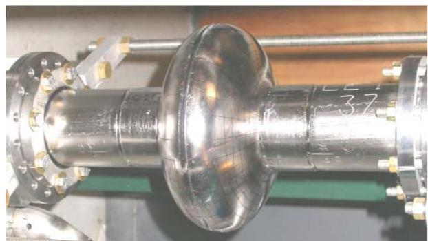
Figure 4: First large-grain niobium single-cell cavity at Cornell. It has Cornell/CEBAF shape. Large-grain disks manufactured by OTIC (Ningxia, China).
