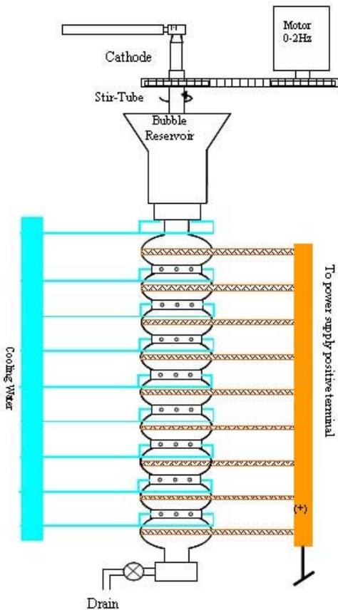
Figure 2: Laout of the vertical EP system
