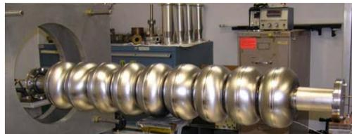
Figure 5: 9-cell re-entrant cavity
