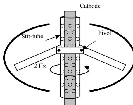
Figure 1. Cathode and stir-tube assembly for one cell. All other cells are identical.
