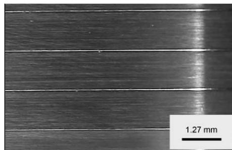
Figure 1: Photograph of HGI surface (R213). The thin horizontal lines are stainless steel layers, while the remainder of the structure is Rexolite.
