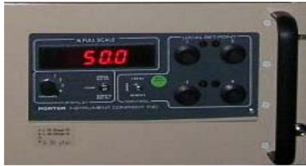
Figure 4: Four-channel flow-control module.
