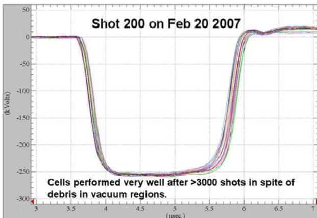
Figure 7. Cells 9-31 were fired at 250 kV for 200 shots at the conclusion of the Scaled Accelerator Tests.
