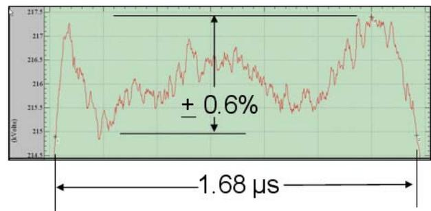
Figure 4b. The average cell voltage on the Scaled Accelerator Test exceeded the design goal of flatness to  $\pm 1.0\%$ .
