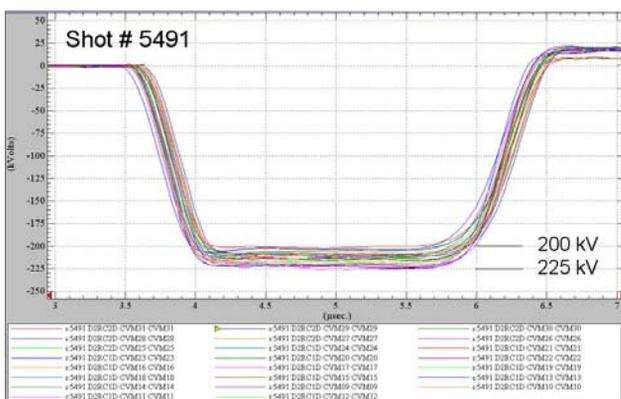
Figure 6. The 24 refurbished cells operated between 200 and 225 kV.
