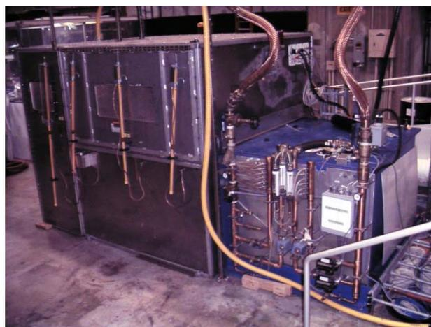
Figure 4: 15 MW output converter-modulator
