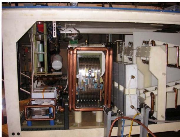
Figure 2: View of doubler capacitors and output filter choke
