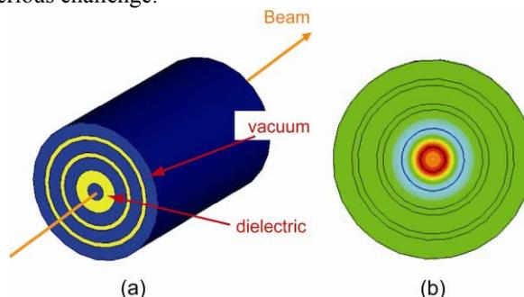
Figure 1: The schematic of an omniguide, the blue area is vacuum and the yellow area is dielectric (a); the longitudinal electric field magnitude in the  $TM_{01}$ -like mode of an omniguide computed with Microwave Studio [6] (b).
