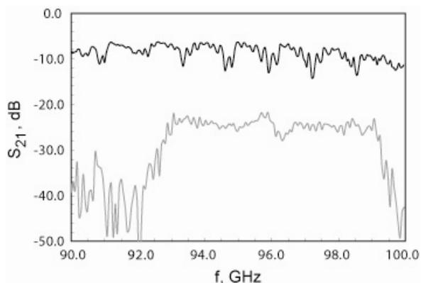
Figure 5: Measured transmission through the omniguide structure (black line). For comparison measured transmission through the LANL W-band vane-loaded TWT structure [3] is shown (grey line).
