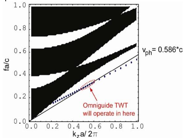
Figure 2: The eigenfrequency of the  $TM_{01}$ -like mode of a  $SiO_2$  omniguide plotted versus the longitudinal wave vector. The dependence is plotted with dots on top of the band gap diagram: black area corresponds to the range of frequencies where the eigenmode cannot be confined inside an omniguide, white area corresponds to the mode confinement region.
