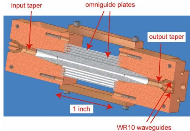
Figure 3: CAD drawing of the omniguide TWT structure and copper couplers.
