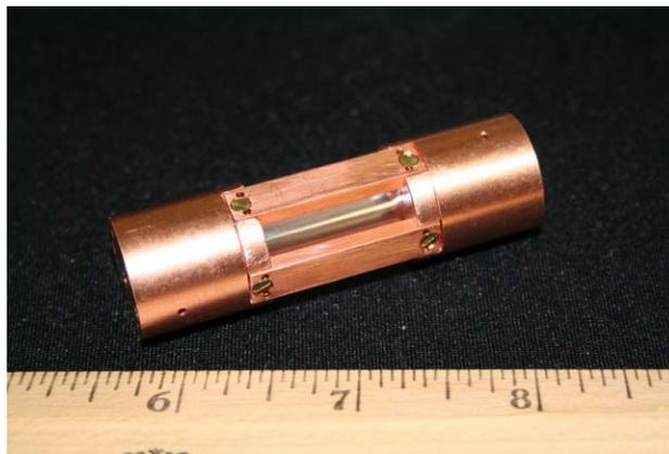
Figure 6: Omniguide TWT structure fabricated for testing with an electron beam (photograph).
