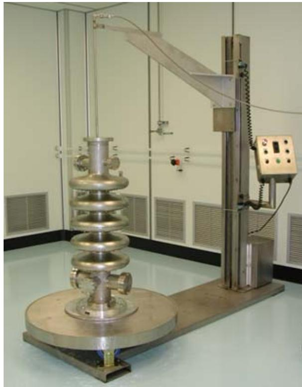
Figure 1: Automatic cavity rinsing station.
