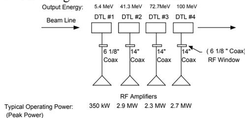
Figure 1: Overview of the 201 MHz RF System Layout.
