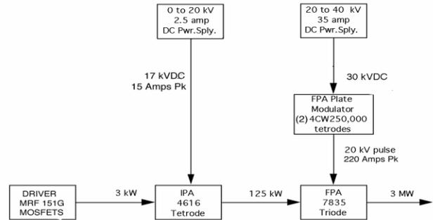
Figure 2: Schematic of the 201 MHz RF Amplifiers.
