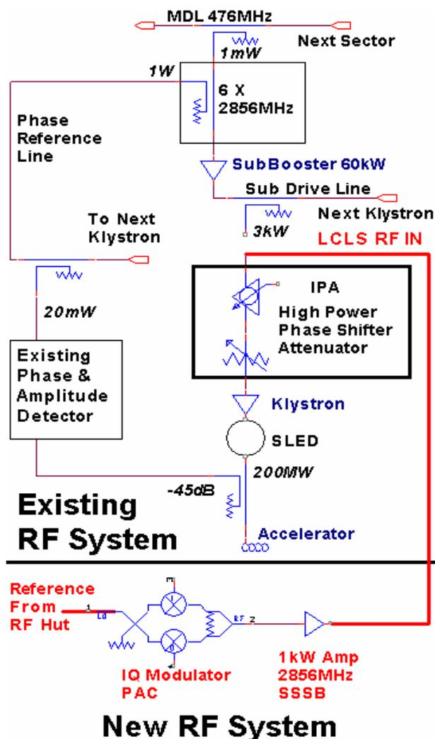
Figure 4: SLAC linac RF system and LCLS input.
