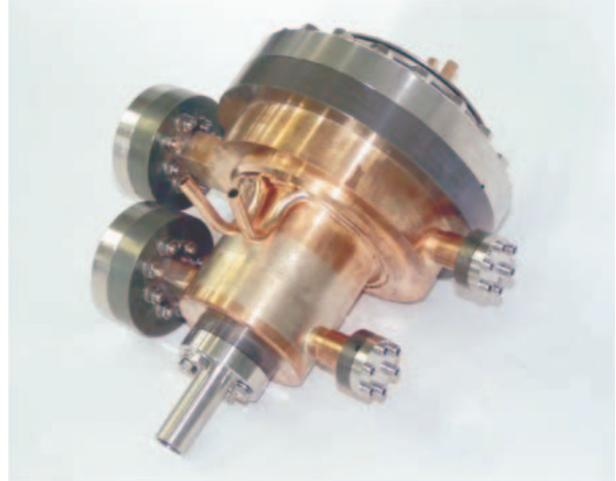
Figure 3: Picture of the pulsed heating cavity awaiting installation.
