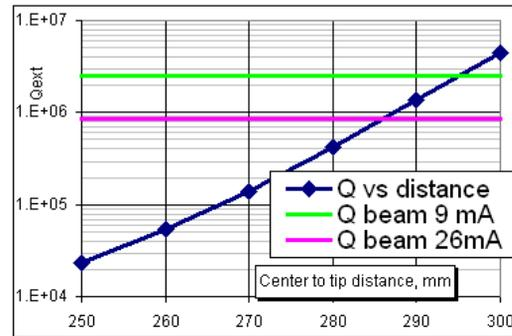
Figure 5:  $Q_{ext}$ : Triple Spoke Cavity.  $\beta=0.62$ , 79mm port.
