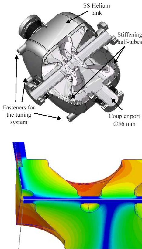
Figure 1: Spoke Cavity and a coupler simulation.
