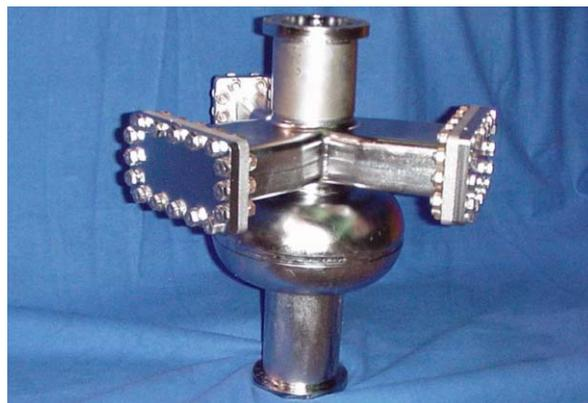
Figure 3: Single Cell Cavity with End Group.
