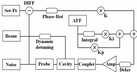
Figure 1: Schematic diagram of the RF control model
