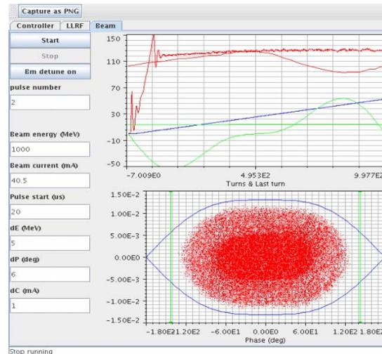
(b) Beam tab—RF power and beam phase space
