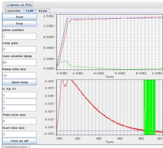
Figure 3: RF control with a loop bandwidth of 10 kHz
