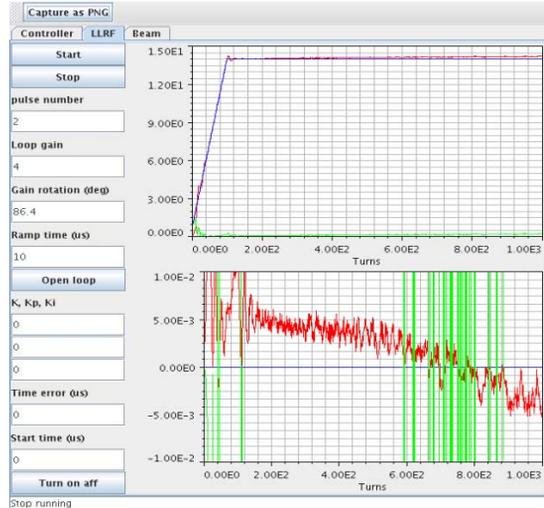
(a) Low-Level RF tab—RF voltage and phase
