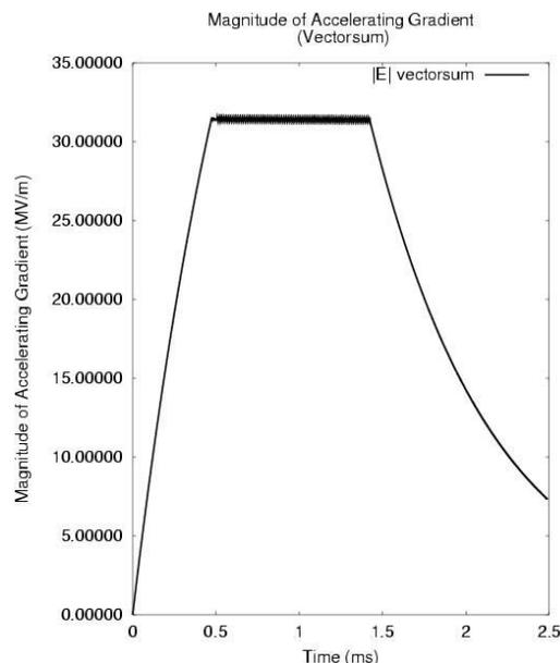
Figure 1: ILC RF pulsed operation with beam. The thicker line at the flattop is gradient fluctuations due to beam.
