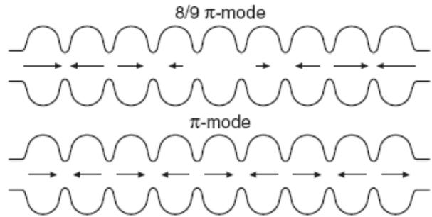
Figure 3: Illustration of the two passband modes included in the simulation, the  $\pi$  mode at 1.3 GHz and the  $8/9\pi$  mode at 1.2992 GHz.
