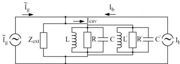
Figure 2: Thomas Schilcher's model of the cavity, with the new addition of an  $8/9\pi$  mode.
