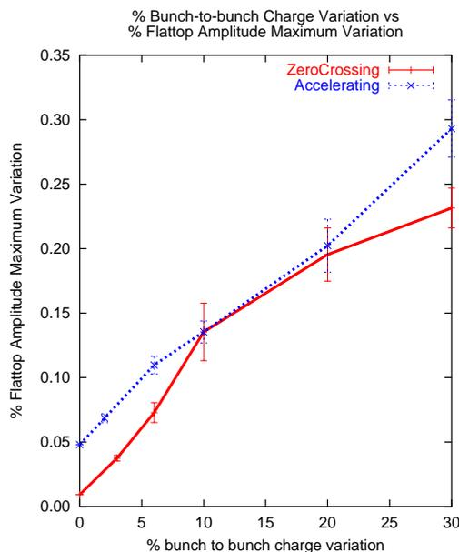
Figure 5: Summary of the RMS fluctuation in bunch-to-bunch charge and the maximum fluctuation in flattop amplitude. Error bars on each point give the range of 5 runs.
