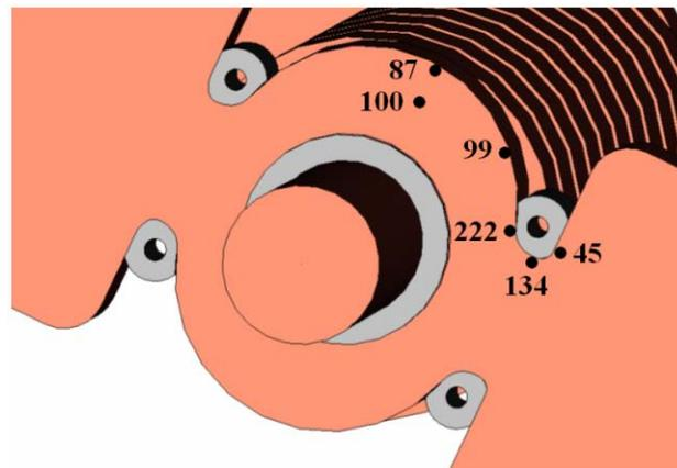
Figure 5: Racetrack cavity configuration showing the normalized values of the magnetic field, the copper heat sink holes, and the stainless steel brazed inserts forming the asymmetrically radiused lips of the coupling apertures.
