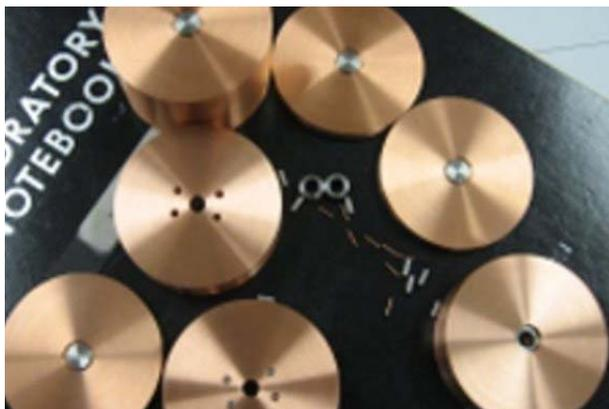
Figure 6: Mixed metal billets being prepared for nickel alloy brazing prior to preliminary and final machining.
