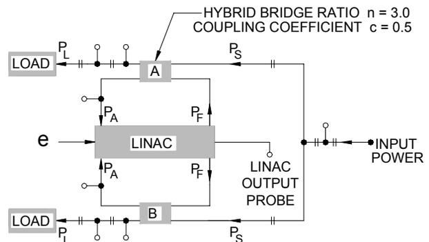
Figure 2: 4X Power amplifier dual recirculating rings with an embedded 17GHz linac test structure.
