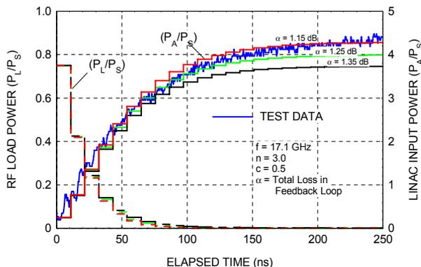
Figure 3: 4X Power buildup and load power decay during successive recirculations.
