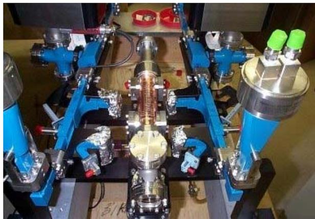
Figure 4: 17GHz linac all-copper structure in the 4X peak power amplifier system.
