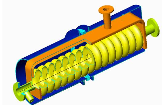
Figure 1: 15-cell SC TW structure with a waveguide inserted into the liquid helium volume.
