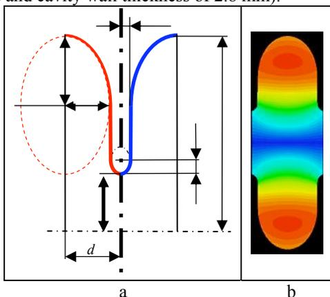
Figure 2: Cell geometry of the superconducting TW accelerating (STWA) structure: (a) STWA structure cavity shape; (b) magnetic field distribution in the STWA cell.
