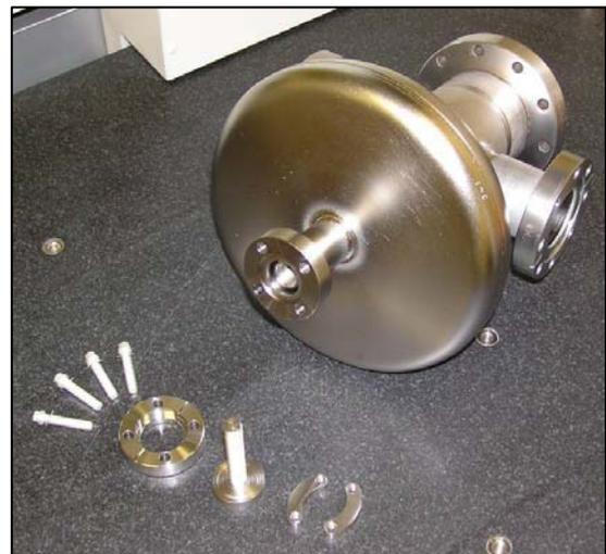
Figure 1. The 1.3 GHz photoinjector with the cathode stalk.
