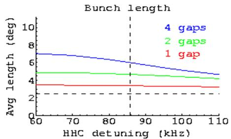
Figure 2: Average bunch length as function of harmonic cavity detuning for NCRF cavities. Total gap is 20% of circumference in each case. Dotted H. line is natural bunch length, V-line optimum short-bunch driven field.
