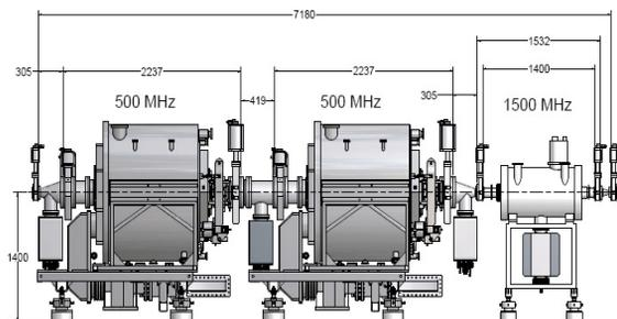
Figure 4: The layout of the RF straight with two fundamental and a single two cell harmonic cavity
