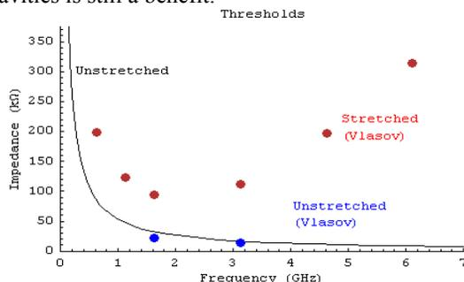
Figure 3: Calculated longitudinal impedance thresholds for stretched and un-stretched bunches.
