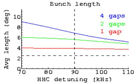
Figure 1: Average bunch length as function of harmonic cavity detuning for SCRF cavities. Total gap is 20% of circumference in each case. Dotted H. line is natural bunch length, V-line optimum short-bunch driven field.
