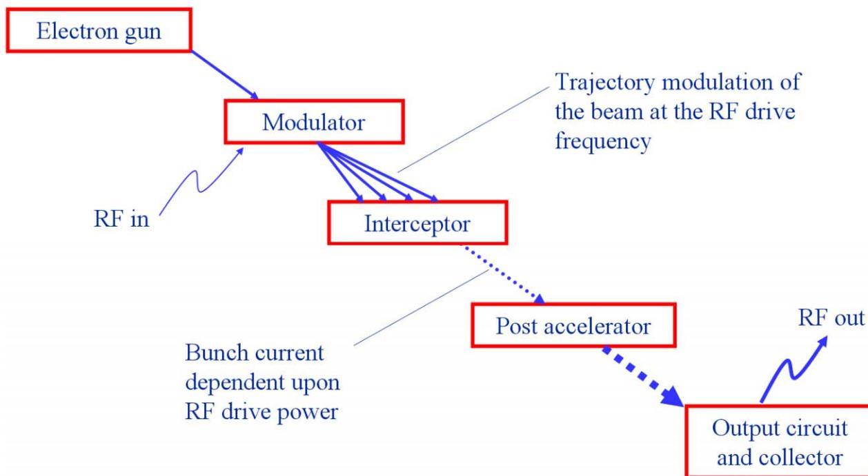
Figure 1: Conceptual layout of the trajectory modulation amplifier.
