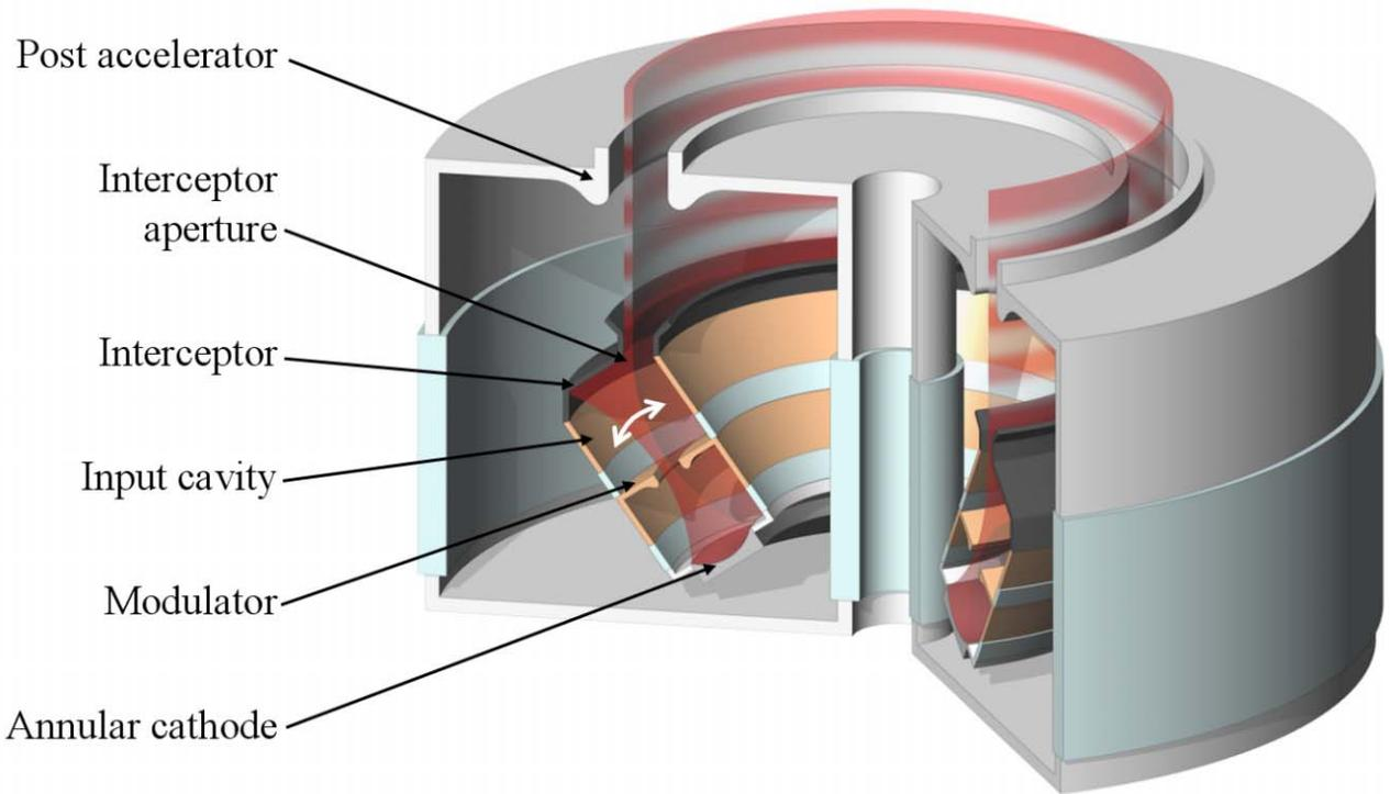
Figure 2: Schematic representation of the integrated input system for the Vector-T™ trajectory modulation amplifier.
