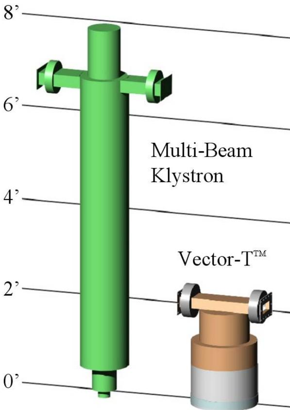
Figure 3: Comparison of approximate dimensions of an ILC-class MBK and the Vector-T™ gridless IOT.
