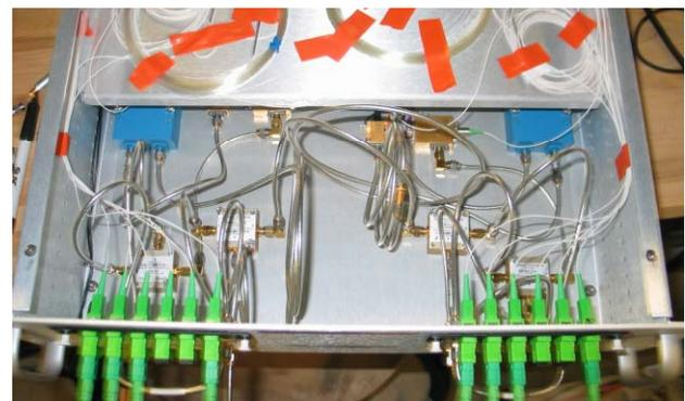
Figure 8: Comb filter chassis.
