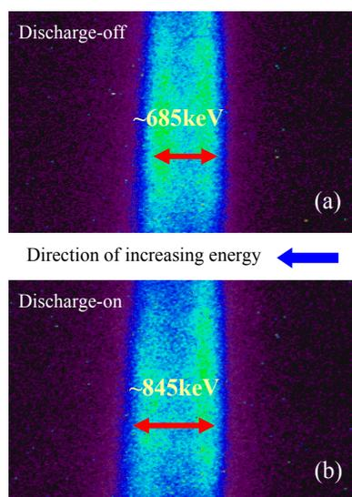
Figure 3: Single-shot electrons beam raw output from the spectrometer with and without discharge in the PASER cell. The horizontal direction corresponds to energy levels increasing from right to left. (a) Raw image without exciting the gas in the PASER cell. Peak-to-peak energy spread of  $\sim$ 685keV is measured. (b) Raw image with the gas excited in the PASER cell. Peak-to-peak energy spread of  $\sim$ 845keV is measured.
