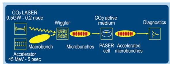
Figure 2: Schematic layout of the PASER experiment. The distance separating the wiggler from the PASER cell is about 2.5m.
