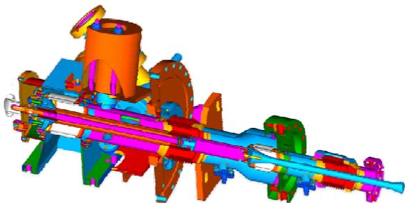
Figure 5: RF input coupler for XFEL.
