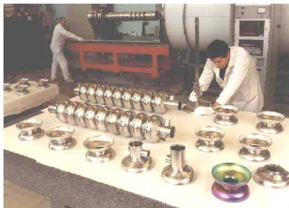
Figure 1: Parts for Nb cavity production: hydroforming Nb sheets and electron beam welding of cavities. (Courtesy CERCA).
