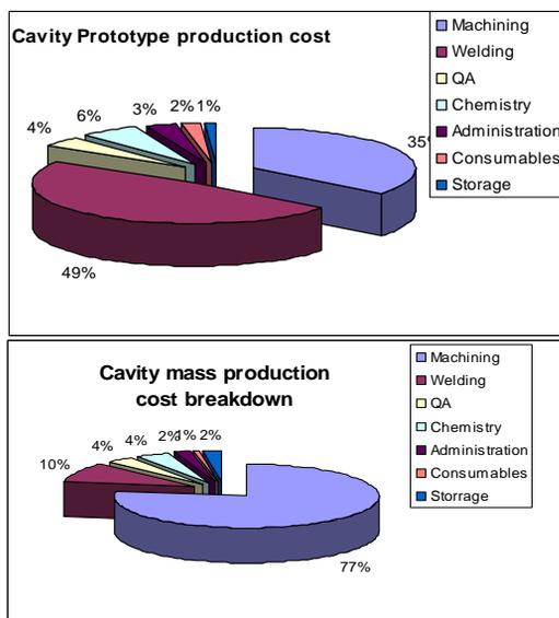
Figure 2: Comparison of cavity fabrication cost breakdown.
