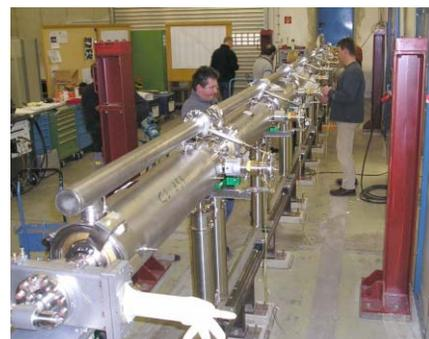
Figure 4: Cavity string assembly for FLASH module.
