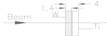
Figure 6: Two-layer target with W as the first one. Dimensions are given in mm
