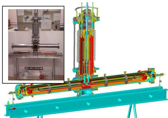
Figure 4: The cross-section of undulator module under assembling in Cornell LEPP. This 1.5 m long prototype model has all elements carried by full 4-m long prototype.
