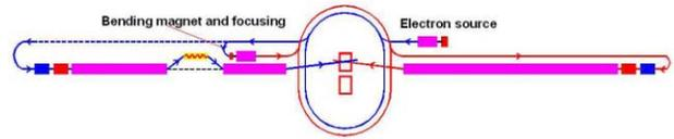
Figure 3: Possible operational scheme for filling positron ring by usage of electron source linac. With stacking and polarized electron source this scheme allows accumulation of polarized positrons.
