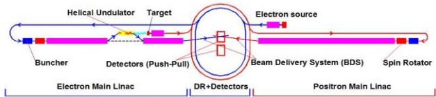
Figure 1: The basic scheme of ILC.
