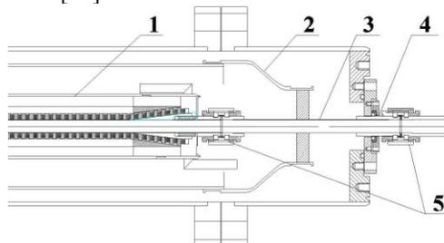
Figure 5: Schematics of transition region between cold mass and the room temperature flange in Cornell undulator. 1—cold mass, 2—70 °K shield, 3—StSteel thin wall tube, 4—Wilson type sealant, 5—Conflat® joints.
