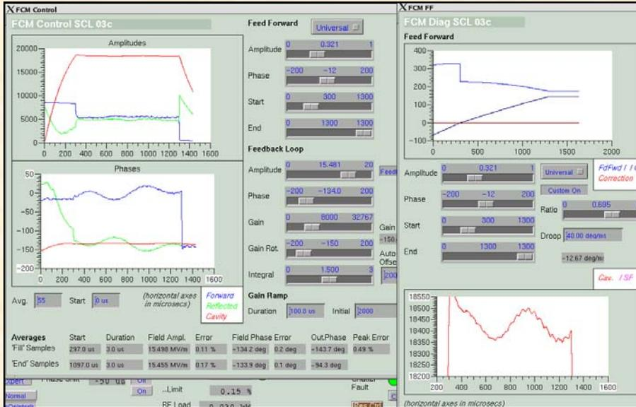
Fig. 1 Adaptive Feed-Forward disabled. Peak field error is 0.5 %.
