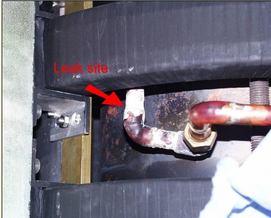
Example of typical water leak on 402.5 MHz klystron.
