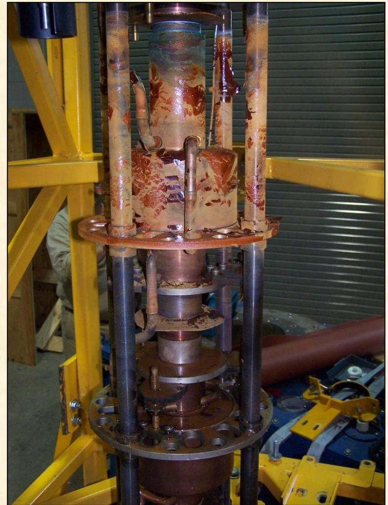
This 805 MHz, 550 kW klystron would not make full power. Upon removal we discovered it was full of water and the input RF connection was submerged!
