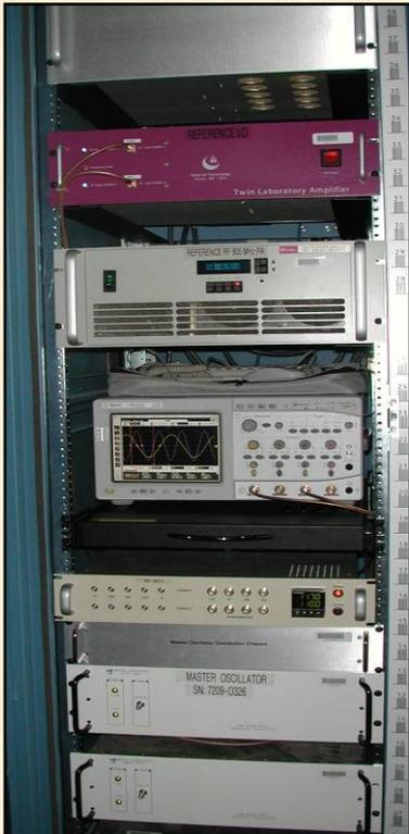
Master oscillator rack located at DTL/CCL transition
