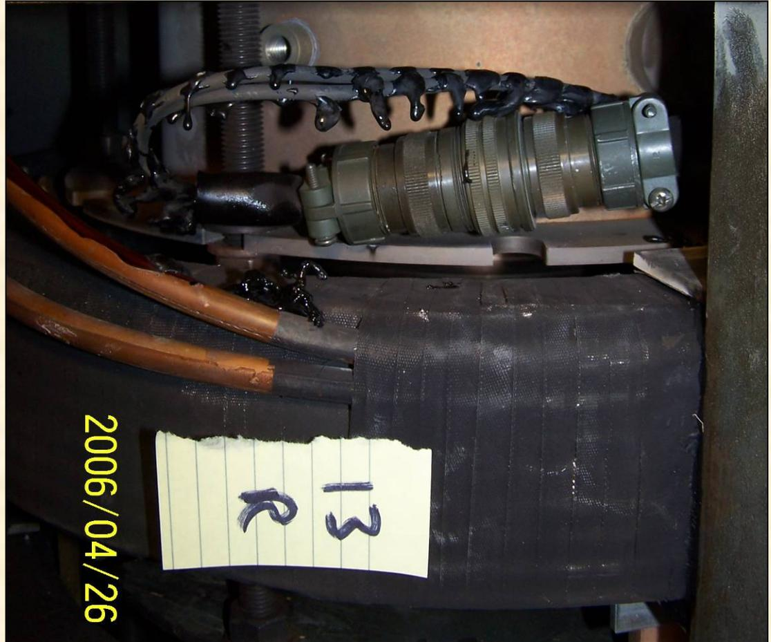
Water leaking onto this solenoid connector caused a short circuit and subsequent arcing and overheating.
