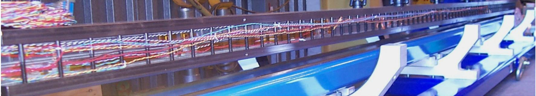
**Assembled shell-yoke structure with dummy coil**
