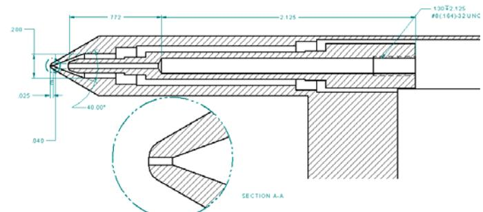
**Carbon beam probe assembly**
