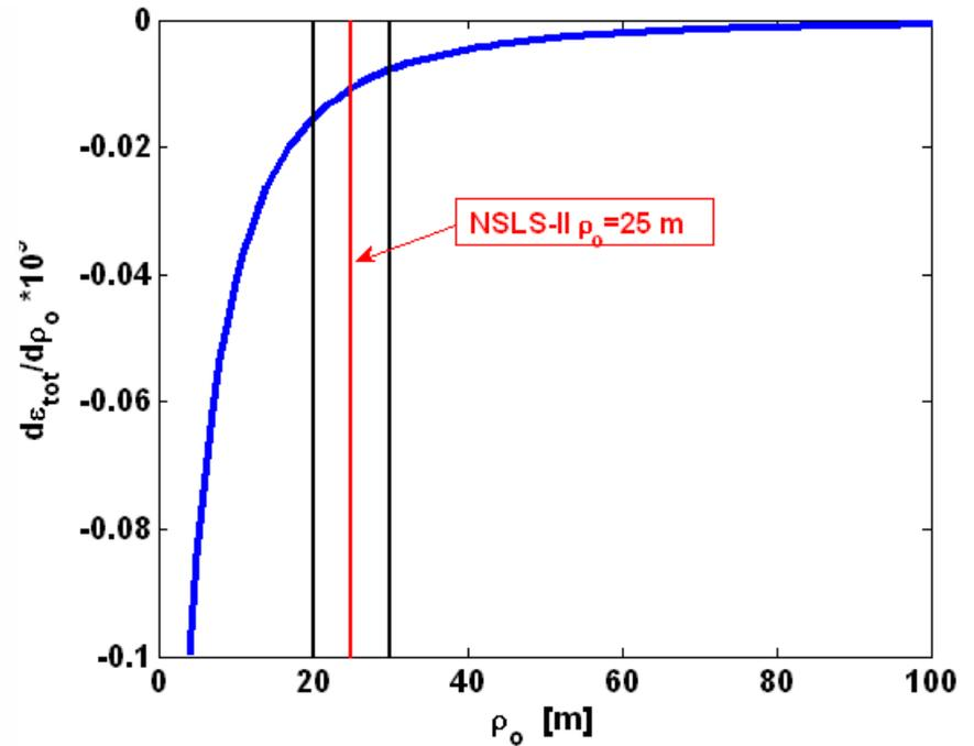
The change of total emittance with IBS growth for 500mA ring current per unit of change of the dipole bend radius. The optimum range is shown, with the NSLS-II value
