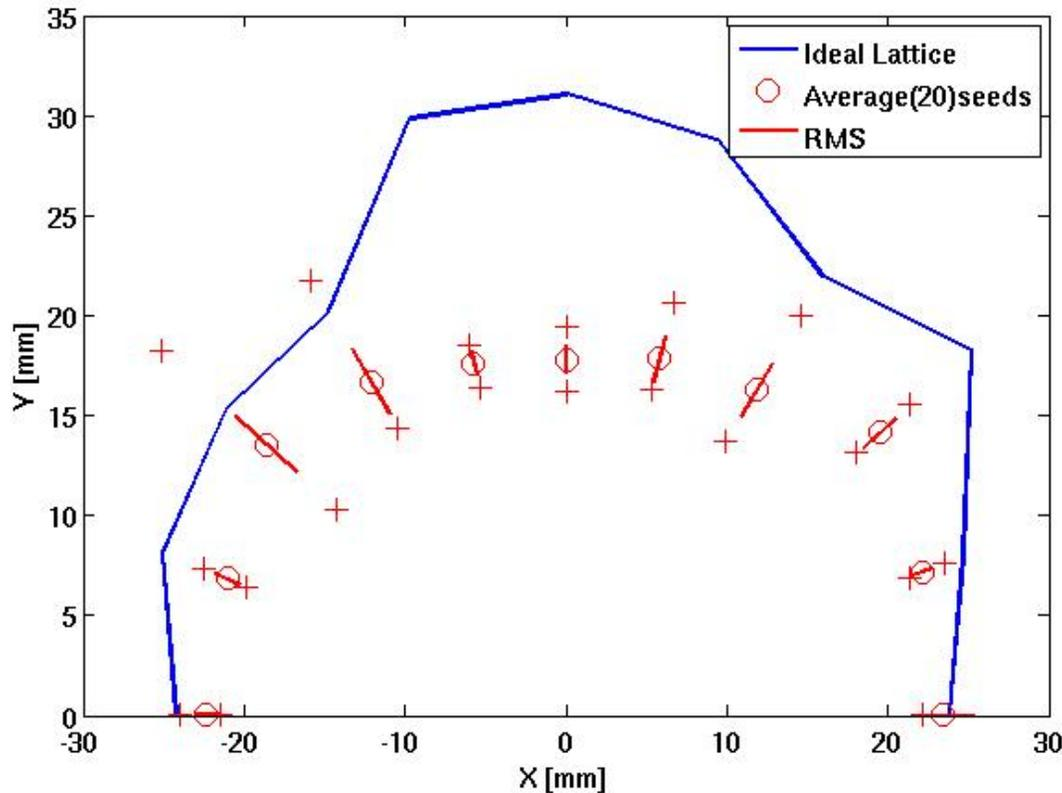
DA is sufficiently robust for the high current operation, complex insertion devices, and top-off injection
